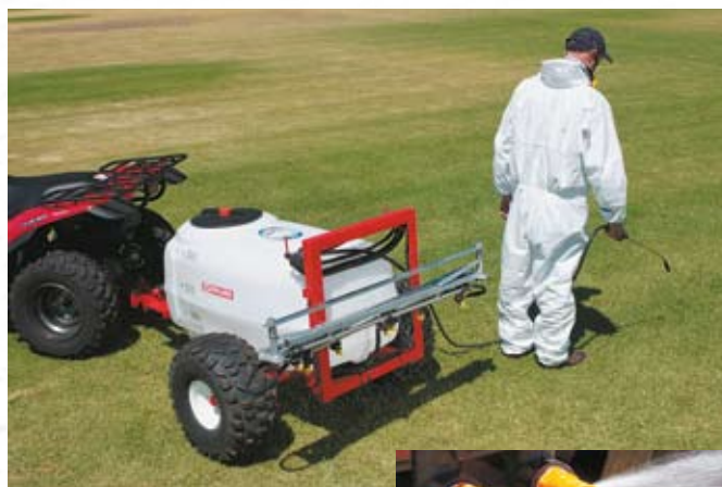
UA300/13/4B shown with boom folded and using spot spray lance.
